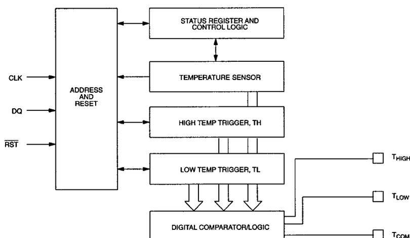
The DS1620 measures temperature using a bandgap-based temperature sensor. The temperature reading is provided in a 9-bit, two's complement reading by issuing a READ TEMPERATURE command. The data is transmitted serially through the 3-wire serial interface, LSB first. The DS1620 can measure temperature over the range of  $-55^{\circ}\text{C}$  to  $+125^{\circ}\text{C}$  in  $0.5^{\circ}\text{C}$  increments. For Fahrenheit usage, a lookup table or conversion factor must be used.
