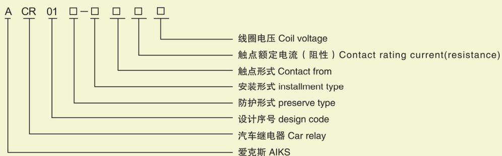
①线圈电压 Coil voltage; DC为直流; DC means direct current;
