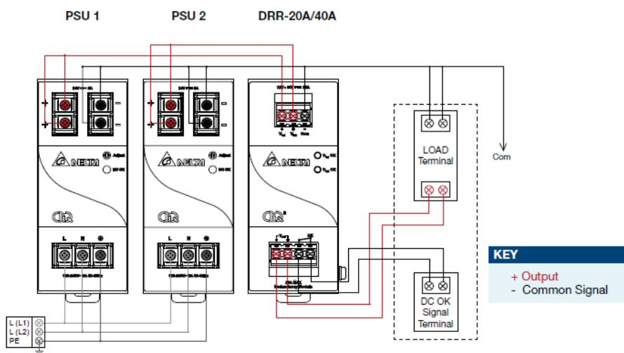
Fig. 2.1 Redundancy / Parallel Operation Connection Diagram
