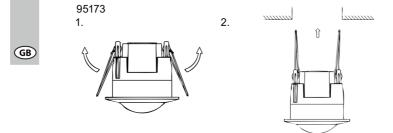
The scope of delivery includes installation material for concrete walls or ceilings. Other materials need other installation material.
