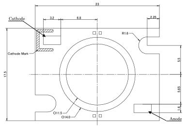
Tolerances unless otherwise specified  $: \pm 0.3$ mm Unit: mm
