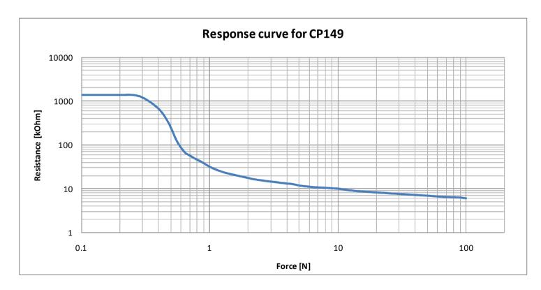
[Response curve depending on actuator shape material and design Measurements performed with a 4mm probe diameter covered with a 2mm thick rubber of 65 Shore A]
