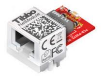
The RJ203 is an "Ethernet front-end" module that contains 10/100BaseT Ethernet magnetics and a standard RJ45 jack. Module's magnetics are designed to work with Davicom's DM9000B Ethernet controller.
