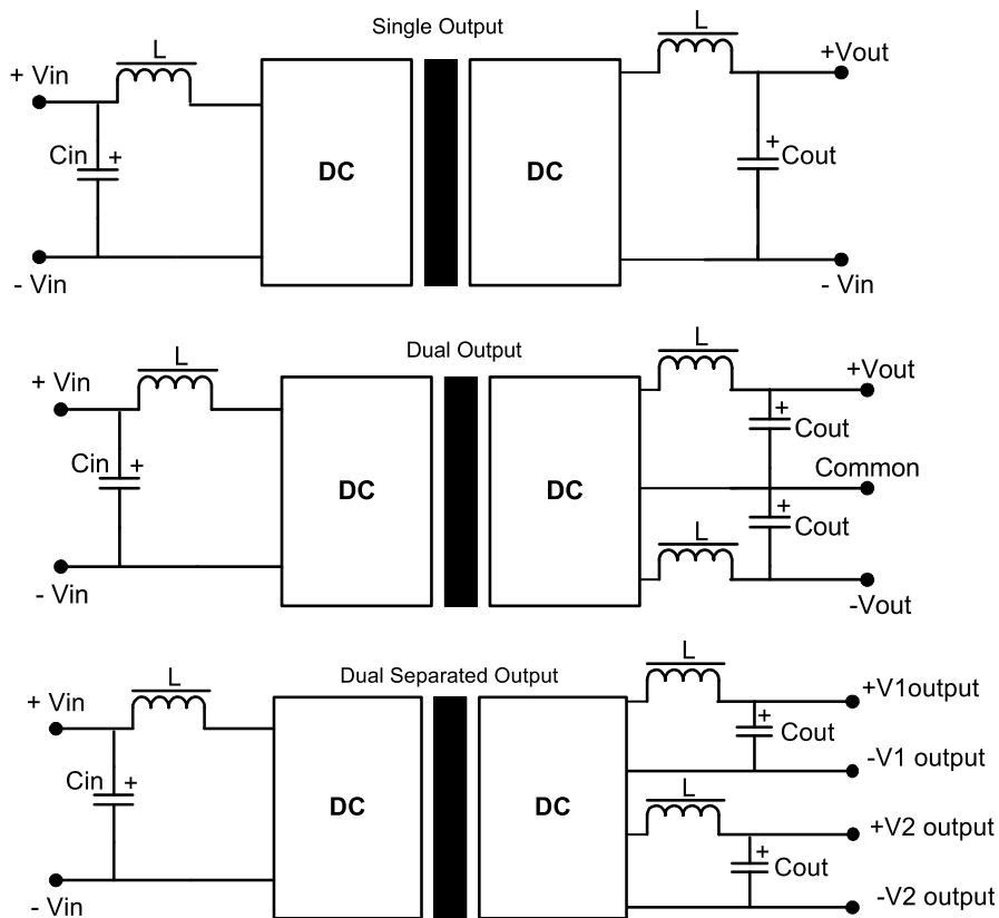
If it is required to decrease the input/output ripple, an "LC" filter network can be installed on the input and output of the converter (see above).
