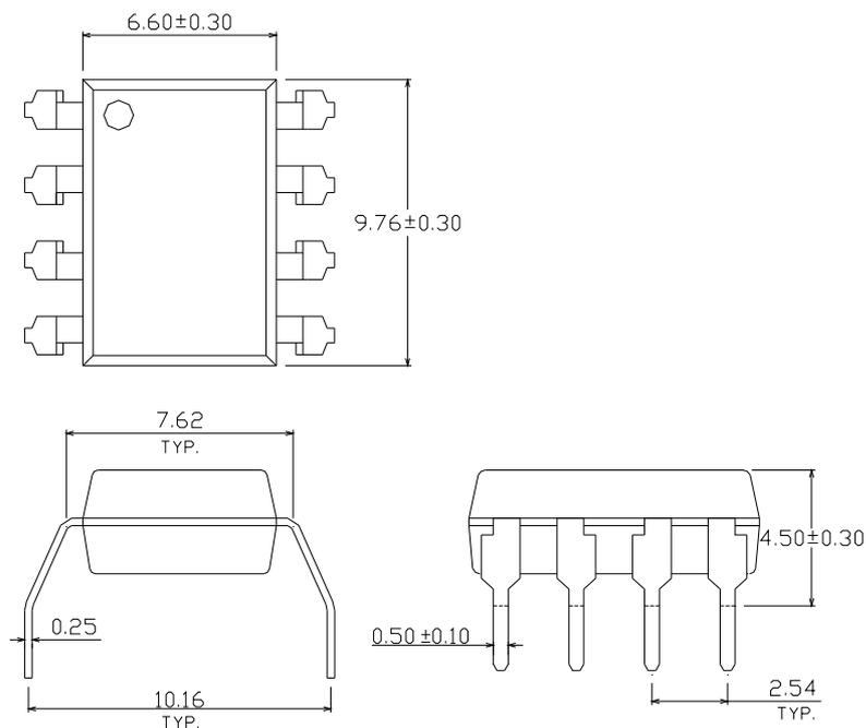
**8 PIN DIP LOW INPUT CURRENT HIGH GAIN
