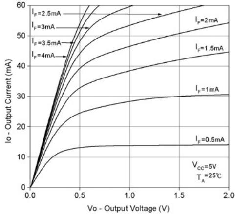
Fig.4 Output Current vs. Input Diode Forward Current
