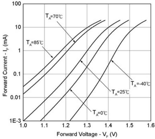
Fig.2 LED Forward Voltage vs. Temperature
