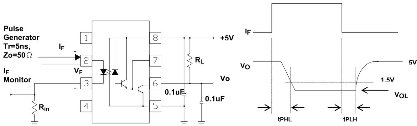
**Fig. 13 Switching Time Test Circuit and Waveform**
