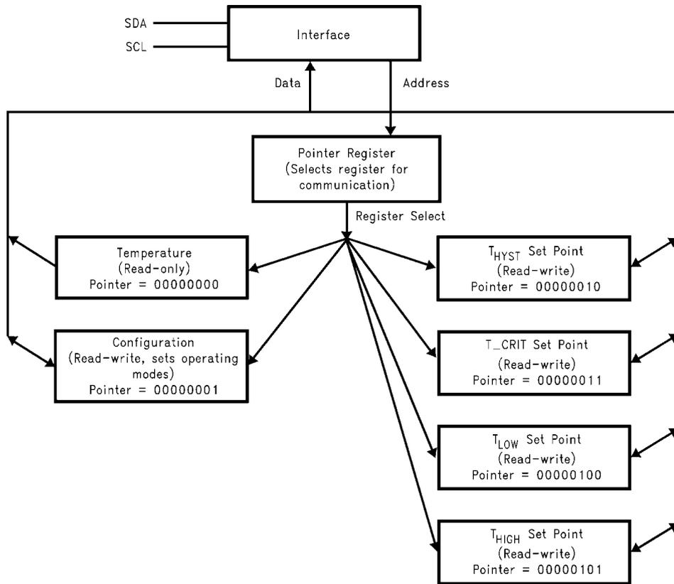
There are four data registers in the LM92, selected by the Pointer register. At power-up the Pointer is set to "00"; the location for the Temperature Register. The Pointer register latches the last location it was set to. In Interrupt Mode, a read from the LM92 resets the INT output. Placing the device in Shutdown mode resets the INT and T\_CRIT\_A outputs. All registers are read and write, except the Temperature register which is read only.
