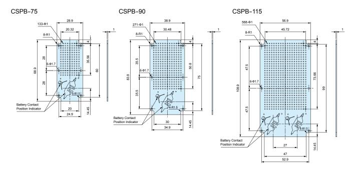
Note : Holes (6- $\Phi$ 1.7) for PCB mount bosses are un-soldered.
