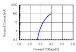
Fig 1. Forward Current vs. Forward Voltage
