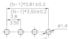
RECOMMEND PCB LAYOUT (TOLERANCE=±0.05)
