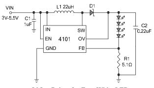
Figure 1. Li-Ion Driver for Four White LEDs
