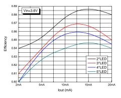
Figure 2. Efficiency vs Number of LEDs
