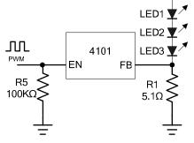
Figure5. Dimming Control Using a PWM Signal
