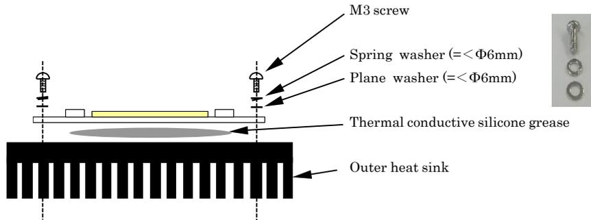
4. A heat radiating grease should be applied to the whole rear surface so that this product can dissipate heat as a whole. This product could be bent during the clamping operation if heat grease in sheet form is used. For this reason, it is recommended that grease in paste form is used.
