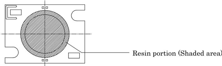
3. This product should be secured firmly by fastening an M3 screw on both sides of the product. Please be careful not to apply any stress to the product during the clamping operation. As the connection status could vary depending on materials of outer heat sink, please check thoroughly.
