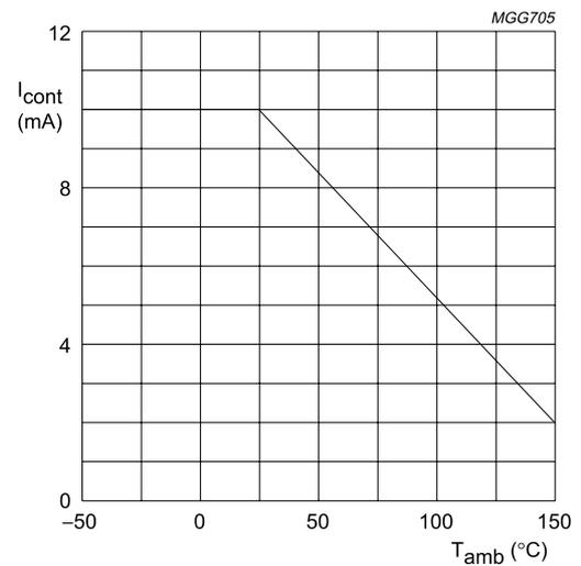
Fig.5 Maximum operating current for safe operation.
