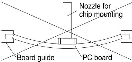
It is recommended that the PC board should be held by means of some adequate supporting pins such as shown left to prevent the SMDs from being damaged or cracked.
