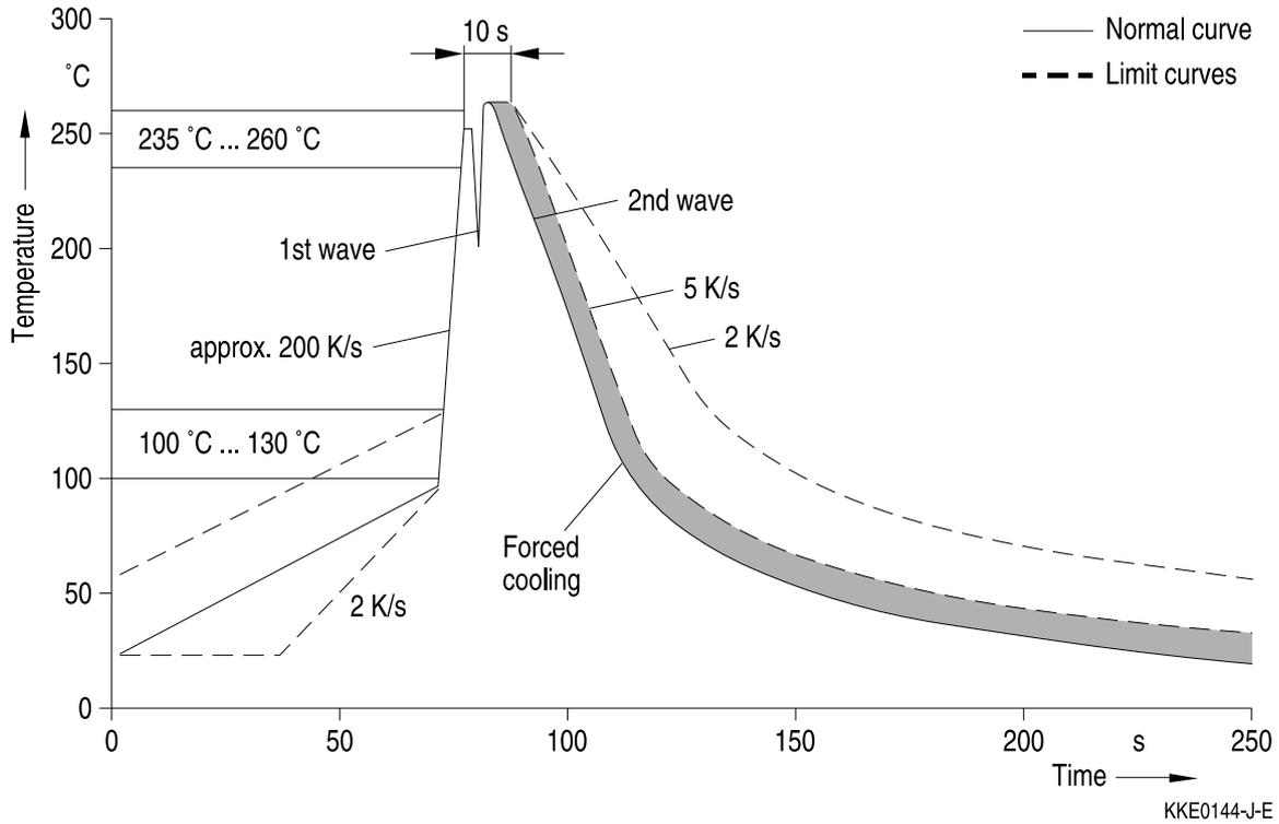
**Solder joint profiles for silver/nickel/tin terminations**
