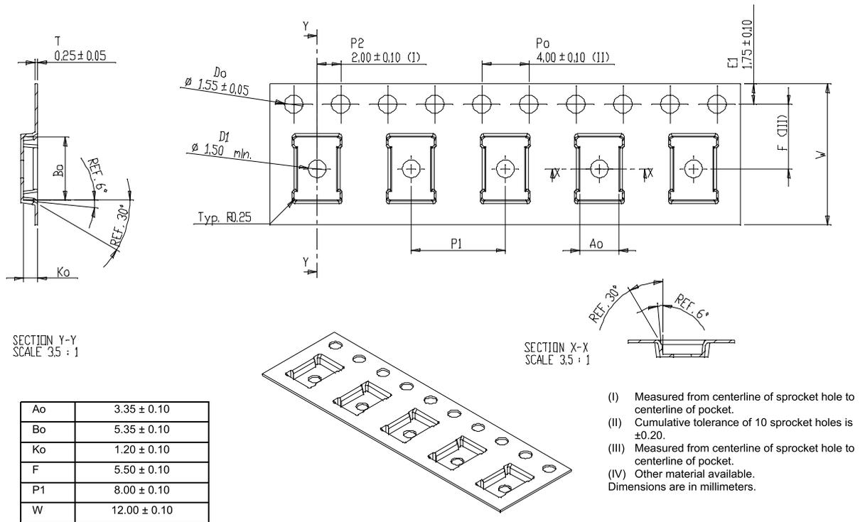
Figure 7. LGA (3 by 5) Embossed Carrier Tape Dimensions
