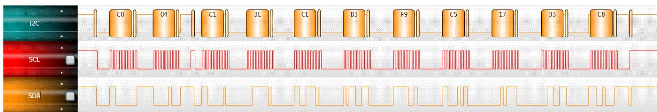
**Figure 3. I<sup>2</sup>C Read Coefficient Datagram**
