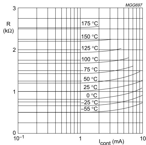
To keep the temperature error low, an operating current of  $I_{cont} = 1 \text{ mA}$  is recommended for temperatures above 100 °C.
