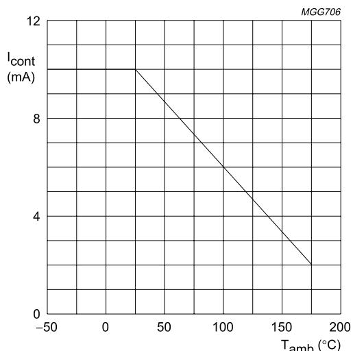
Fig.5 Maximum operating current for safe operation.
