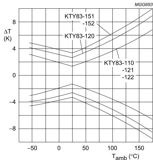
Fig.2 Maximum expected temperature error ( $\Delta T$ ).
