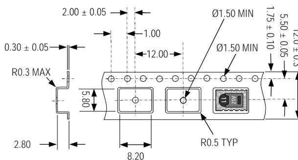
**Figure 21:** Tape configuration and unit orientation within tape, dimensions in mm (1mm = 0.039inch). The leader tape is at the right side of the figure while the trailer tape is to the left (direction of unreeling).
