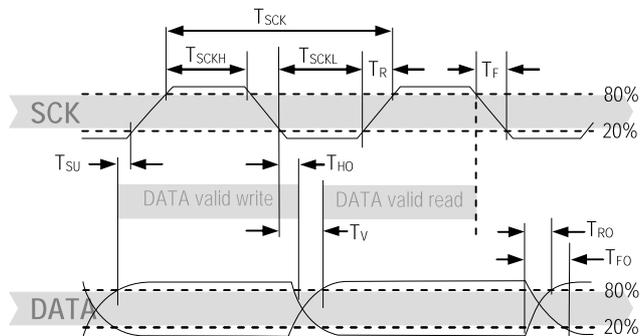
**Figure 11:** Timing Diagram, abbreviations are explained in Table 3. Bold DATA line is controlled by the sensor, plain DATA line is controlled by the micro-controller. Note that DATA valid read time is triggered by falling edge of anterior toggle.
