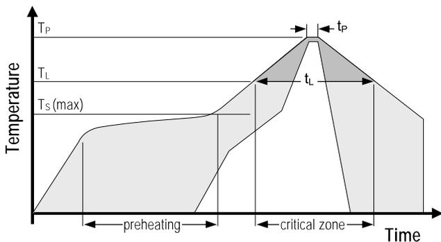
Figure 5: Soldering profile according to JEDEC standard.  $T_P \leq 260^\circ\text{C}$  and  $t_P < 40\text{sec}$  for Pb-free assembly.  $T_L < 220^\circ\text{C}$  and  $t_L < 150\text{sec}$ . Ramp-up/down speeds shall be  $< 5^\circ\text{C}/\text{sec}$ .
