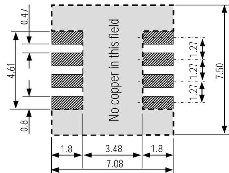
Figure 7: Recommended footprint for SHT1x. Values in mm.
