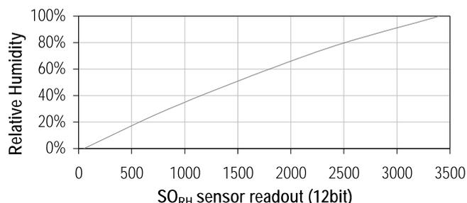
**Figure 18:** Conversion from SO<sub>RH</sub> to relative humidity
