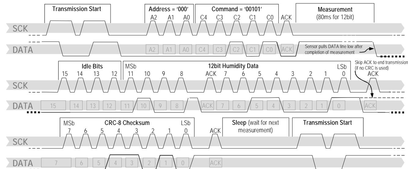
Figure 17: Example RH measurement sequence for value “0000’0100’0011’0001” = 1073 = 35.50%RH (without temperature compensation). DATA valid times are given and referenced in boxes on DATA line. Bold DATA lines are controlled by sensor while plain lines are controlled by the micro-controller.
