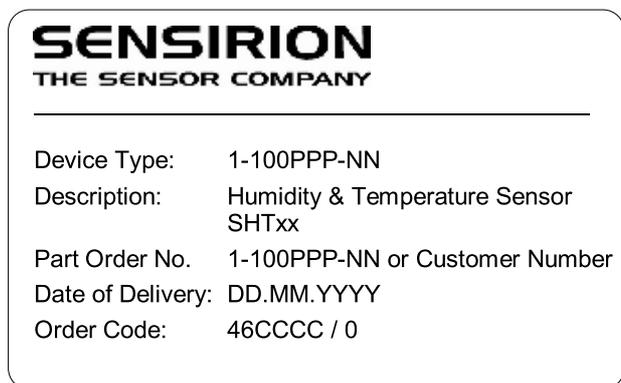
**Figure 20:** Second label on reel: For Device Type and Part Order Number please refer to Table 12, Delivery Date (also Date Code) is date of packaging of sensors (DD = day, MM = month, YYYY = year), CCCC = Sensirion order number.
