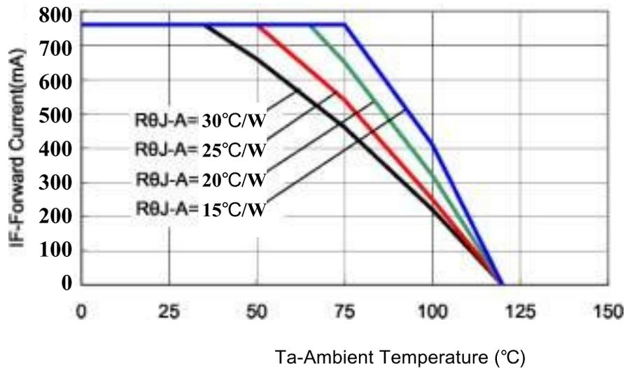
Fig 5b. Maximum Forward Current vs. Ambient Temperature. Derating based on  $T_{jMAX}=120^{\circ}\text{C}$  for Yellow and Red.
