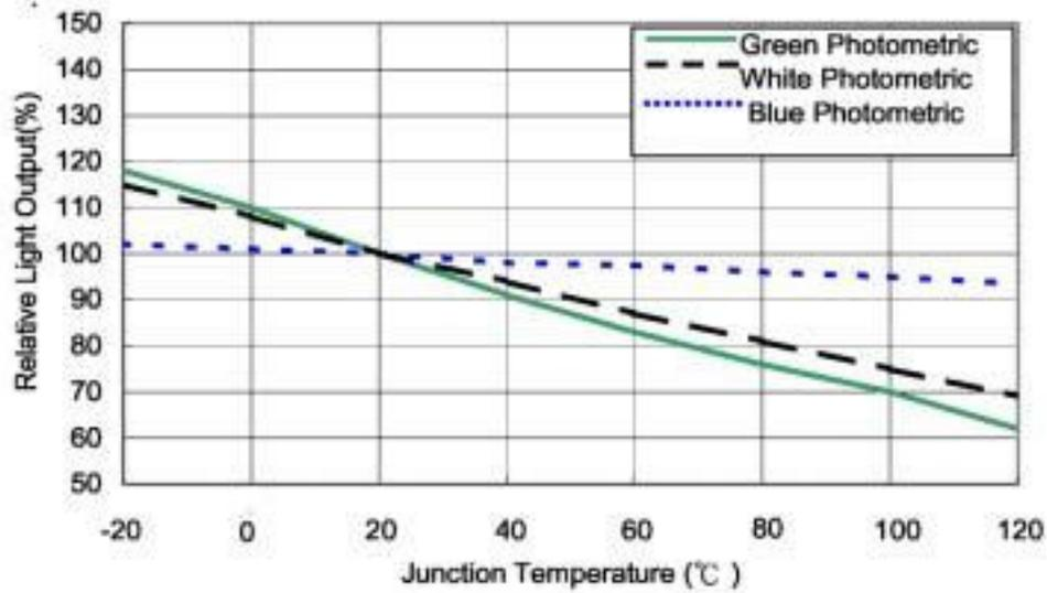
Figure 2a. Relative Light Output vs. Junction Temperature
