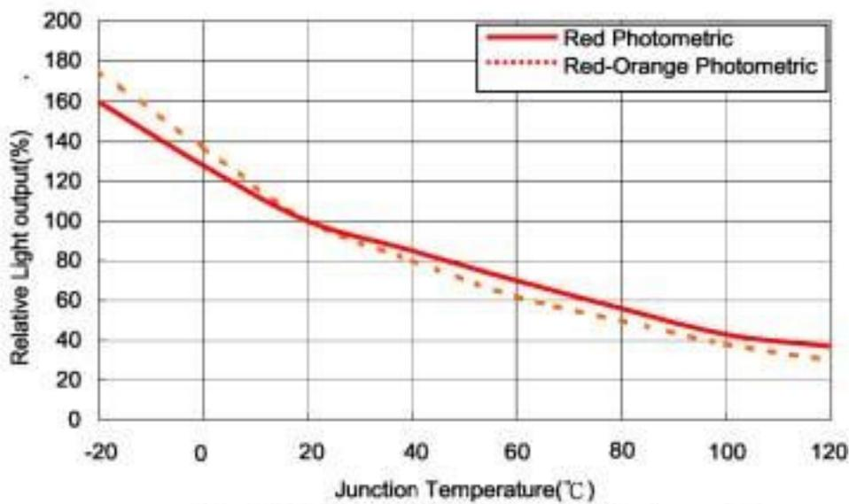
Figure 2b. Relative Light Output vs. Junction Temperature
