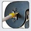
Lateral loading of the cord end sleeve into the clamping position
