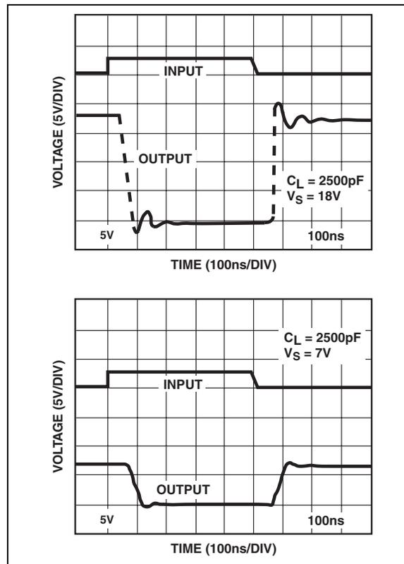
**FIGURE 4-2:** Switching Speed.
