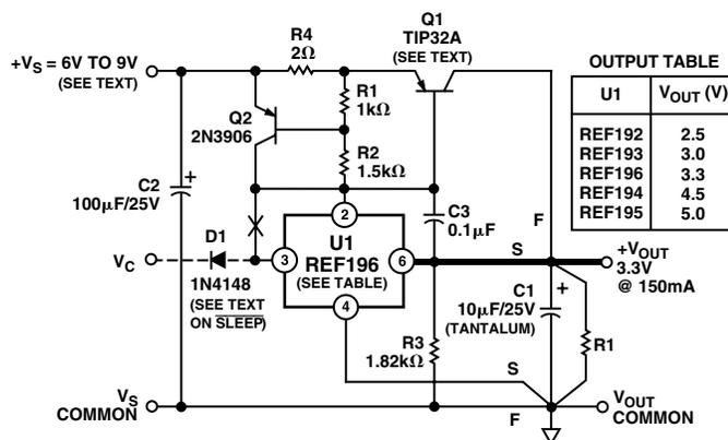
Figure 4. A Boosted 3.3 V Reference with Current Limiting
