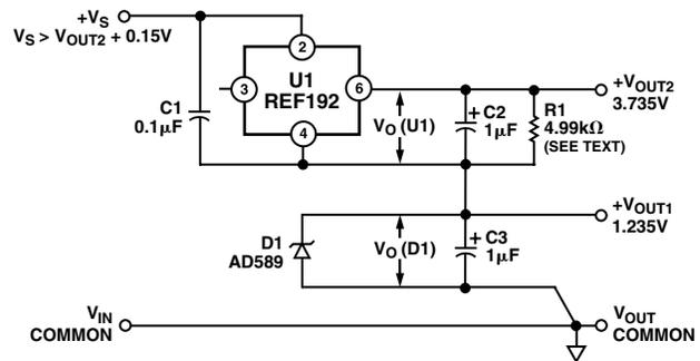
Figure 7. Stacking Voltage References with the REF19x
