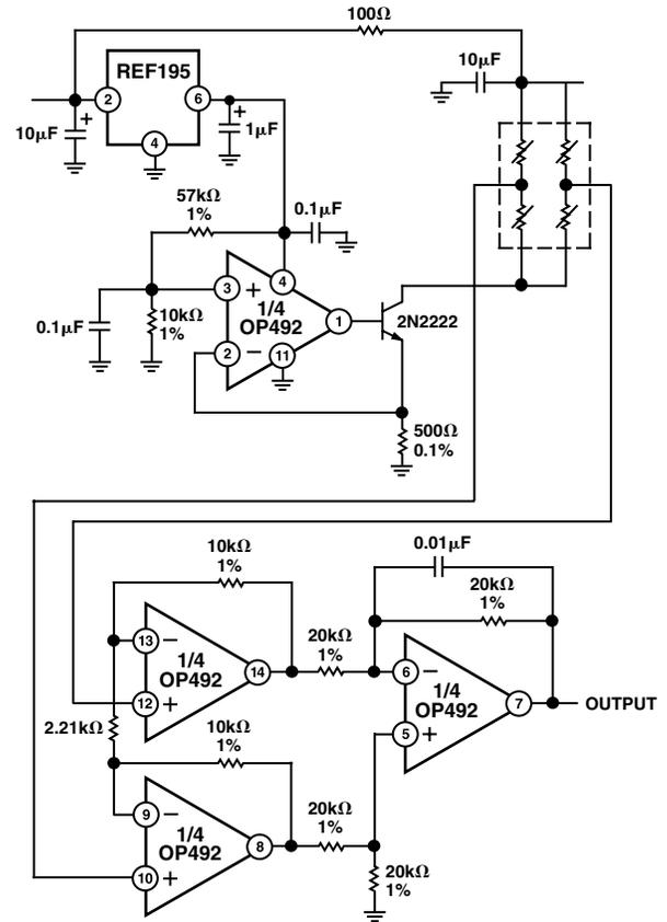
Figure 12. A Low Power, Strain Gage Circuit
