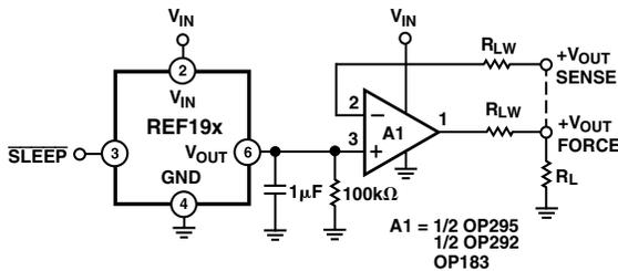
Figure 10. A Low Dropout, Kelvin Connected Voltage Reference
