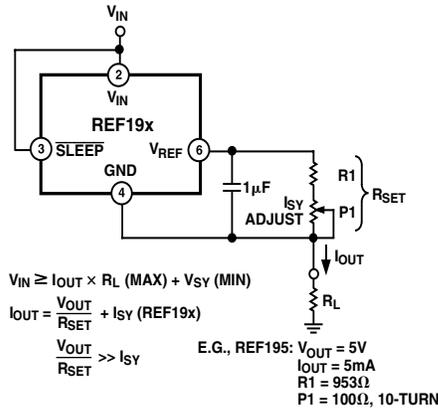
Figure 8. A Low Dropout, Precision Current Source
