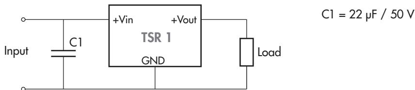
Input filter to meet EN 55022 class A
