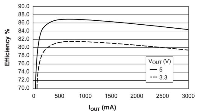
Circuit for 42 V step down to 3.3 V at 3 A. Efficiency data from circuit shown in left panel. Data is for reference only.
