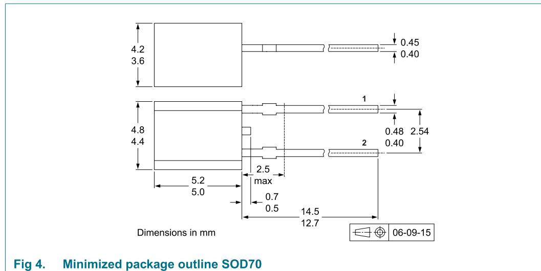
Fig 4. Minimized package outline SOD70
