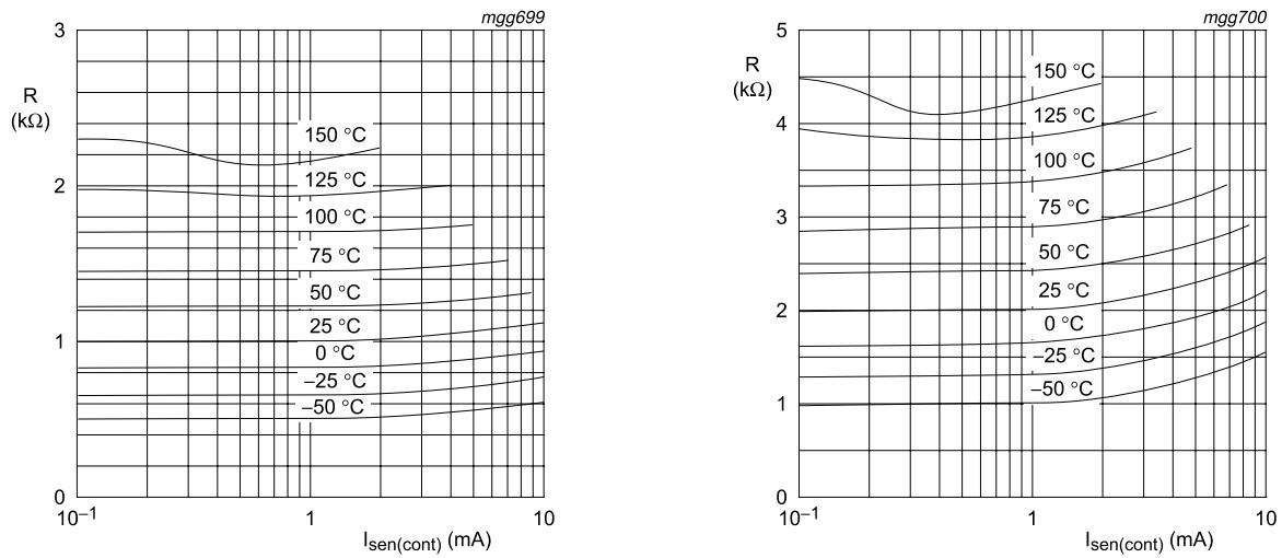
To keep the temperature error low, an operating current of  $I_{\text{sen(cont)}} = 1 \text{ mA}$  is recommended for temperatures above 100 °C
