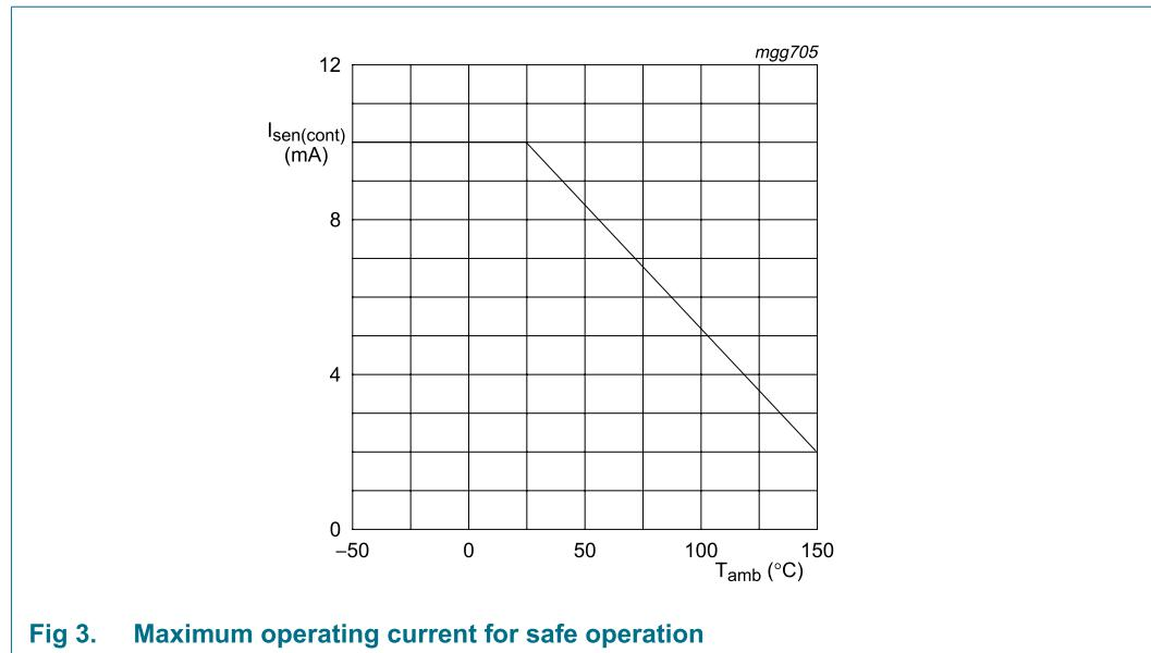
Fig 3. Maximum operating current for safe operation
