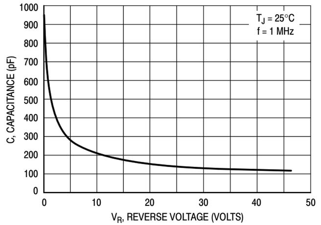
Figure 12. Typical Capacitance
