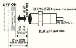
Shift the detected object according to appointed method, from standard position(distance between standard surface to detecting action(rest))
