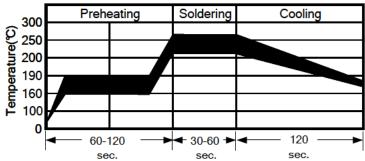
Recommended reflow methods IR, vapor phase oven, hot air oven. Devices are not designed to be wave soldered to the bottom side of the board.
