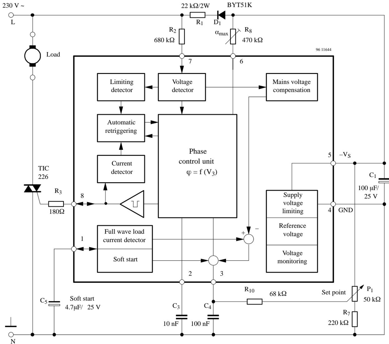
Figure 2. Block diagram with typical circuit: Soft start
