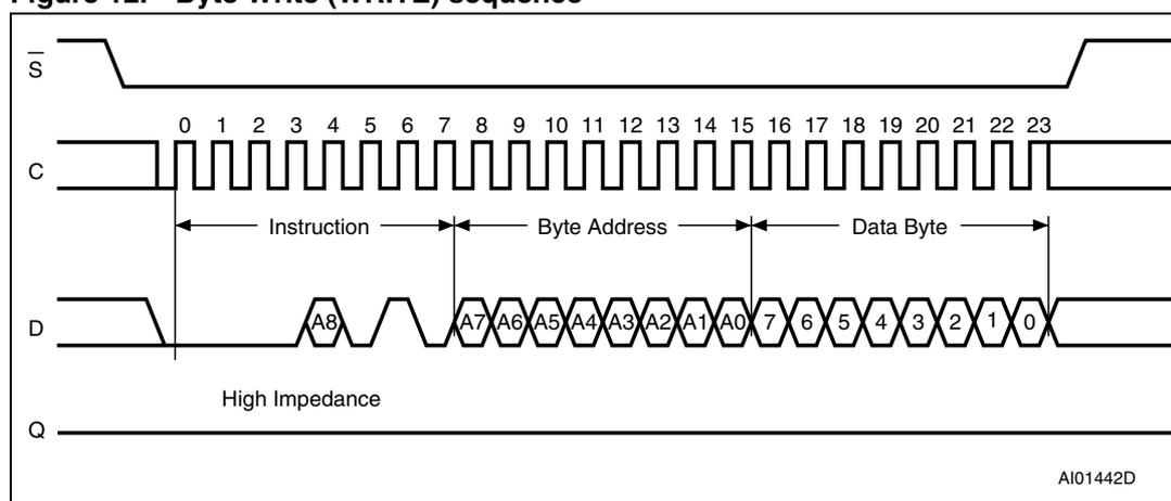
1. Depending on the memory size, as shown in [Table 6: Address range bits](#), the most significant address bits are Don't Care.
