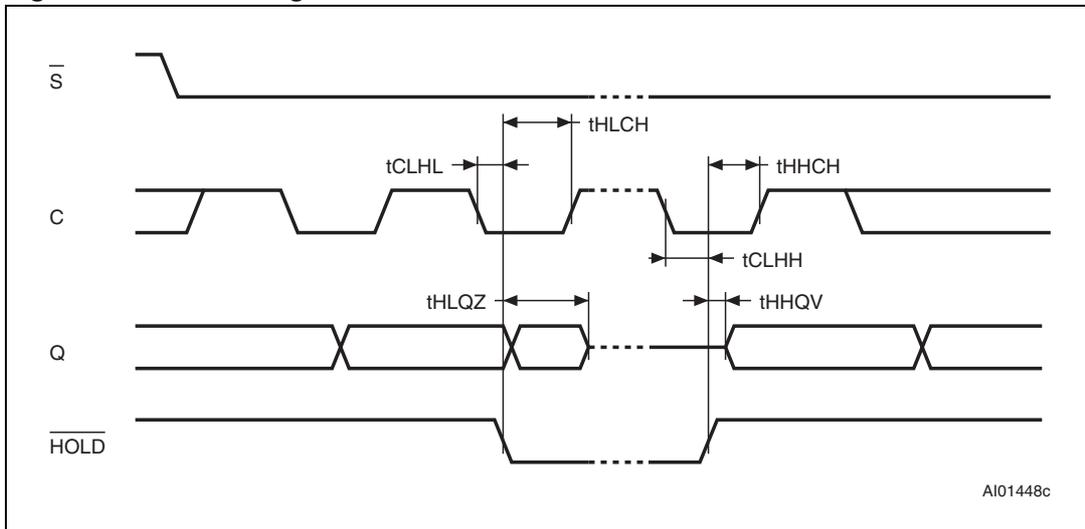
Figure 17. Serial output timing
