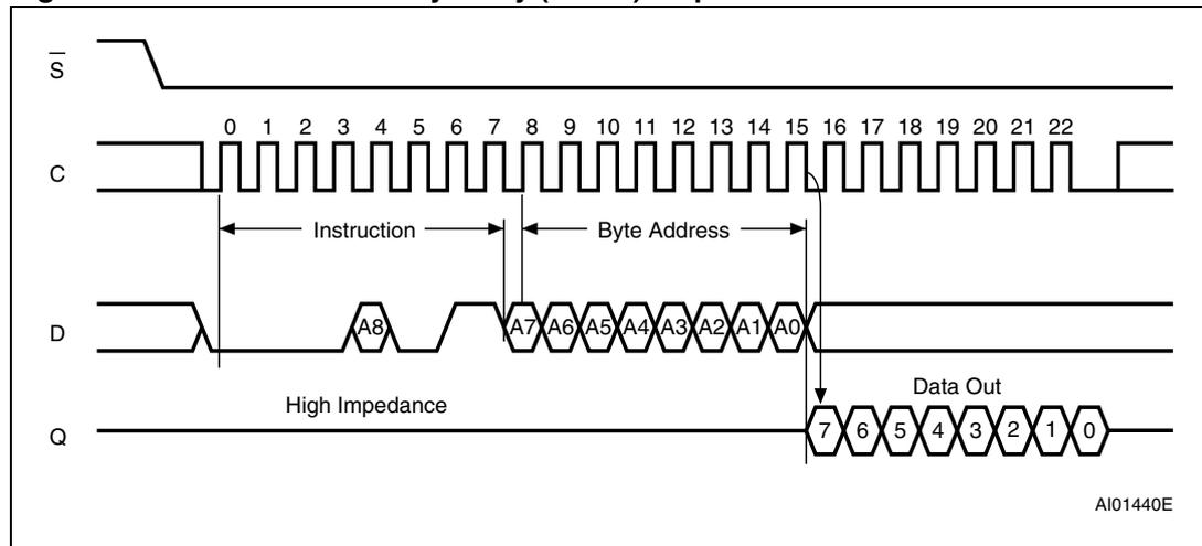
1. Depending on the memory size, as shown in *Table 6: Address range bits*, the most significant address bits are Don't Care.
