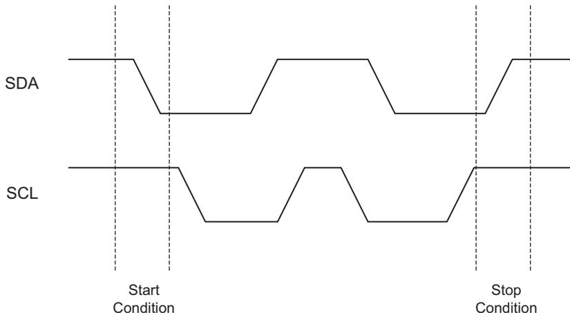
**Stop Condition:** A low-to-high transition of SDA with SCL high is a Stop condition. After a Read sequence, the Stop condition will place the EEPROM in a standby power mode (See [Figure 6-2](#)).
