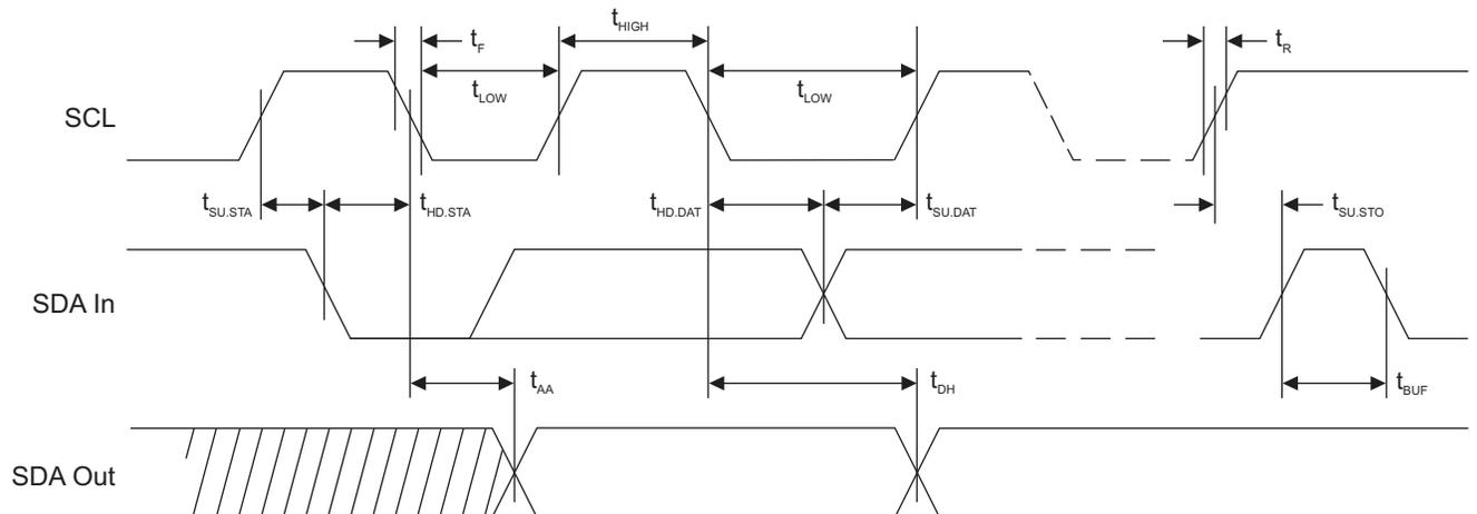
**Figure 6-5. Write Cycle Timing**
