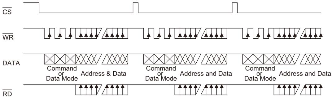
Note: It is recommended that the host controller should read in the data from the DATA line between the rising edge of the RD line and the falling edge of the next RD line.
