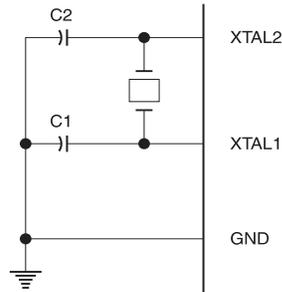
Note: C1, C2 = 5 pF  $\pm$  5 pF for Crystals
