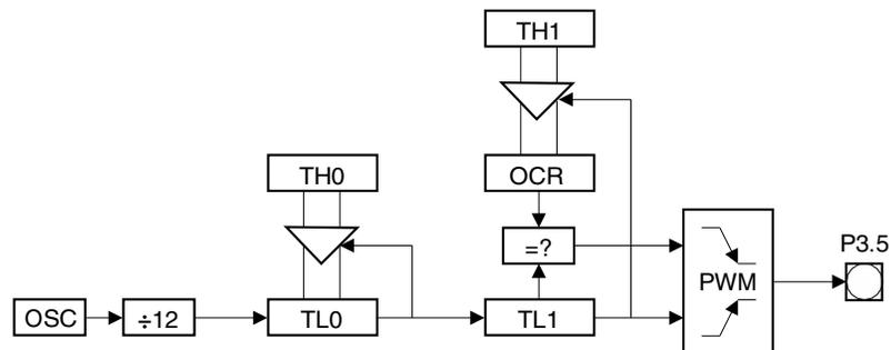
TL0 counts once every machine cycle (1 machine cycle = 12 clocks in X1 mode) and TH0 is the reload value for when TL0 overflows. Every time TL0 overflows TL1 increments by one, with TL0 overflowing after counting 256 minus TH0 machine cycles.
