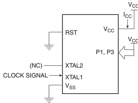
**49.  $I_{CC}$  Test Condition, Idle Mode, All Other Pins are Disconnected**
