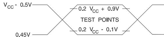
Note: 1. AC Inputs during testing are driven at  $V_{CC} - 0.5V$  for a logic 1 and  $0.45V$  for a logic 0. Timing measurements are made at  $V_{IH\text{ min.}}$  for a logic 1 and  $V_{IL\text{ max.}}$  for a logic 0.
