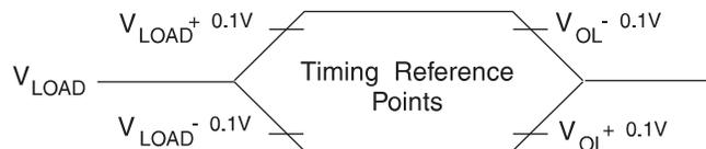
Note: 1. For timing purposes, a port pin is no longer floating when a  $100\text{ mV}$  change from load voltage occurs. A port pin begins to float when  $100\text{ mV}$  change from the loaded  $V_{OH}/V_{OL}$  level occurs.
