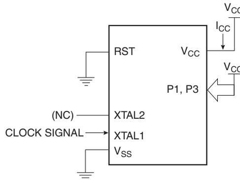
**50. Clock Signal Waveform for  $I_{CC}$  Tests in Active and Idle Modes,  $t_{CLCH} = t_{CHCL} = 5\text{ ns}$**
