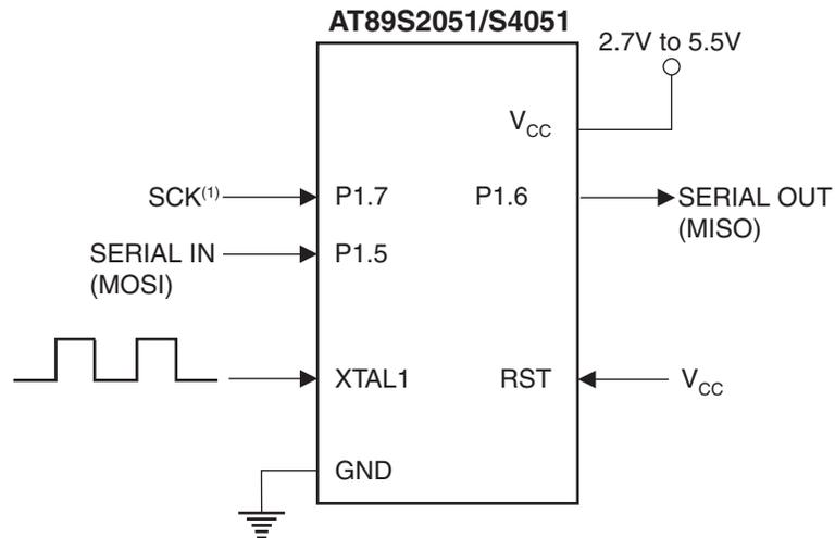
Note: 1. SCK frequency should be less than (XTAL frequency)/8.
