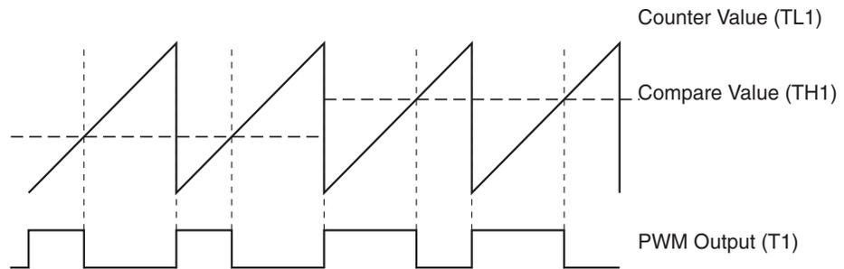
**Figure 16-2.** Timer 0/1 Pulse Width Modulation Mode
