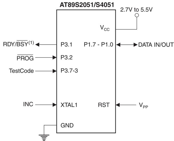
Note: 1. Sampling of pin P3.1 ( $\overline{\text{RDY/BSY}}$ ) is optional. In Parallel Mode, P3.1 will be pulled low while the device is busy. However, it requires an external passive pull-up to  $V_{CC}$ . Also, note that P3.6 does not exist, so TestCode connects to P3.7, P3.5, P3.4, and P3.3.
