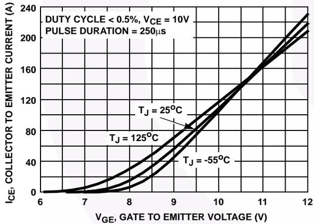
FIGURE 13. TRANSFER CHARACTERISTIC
