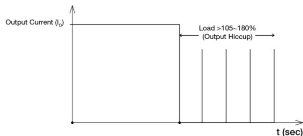
Additionally, if the  $I_o$  is  $<105-180\%$  but  $>100\%$  for a prolonged period of time (depending on the load), the Over Temperature Protection (OTP) will be activated due to high temperature on critical components. The power supply will then go into "Latch-off mode" until the PSU cools down and the AC power is recycled.
