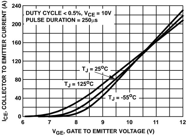
FIGURE 13. TRANSFER CHARACTERISTIC
