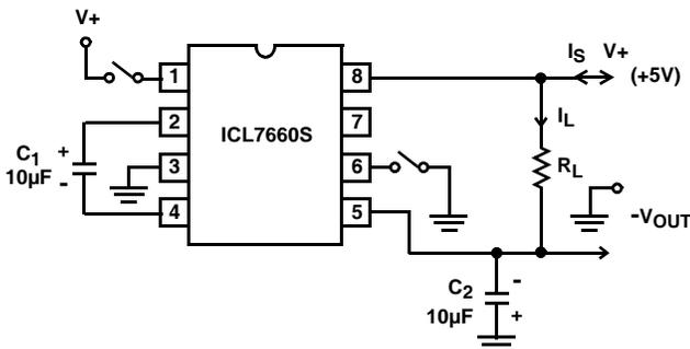
NOTE: For large values of  $C_{OSC}$  (>1000pF) the values of  $C_1$  and  $C_2$  should be increased to 100 $\mu$ F.
