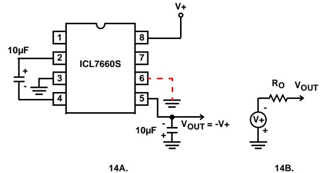
FIGURE 14. SIMPLE NEGATIVE CONVERTER AND ITS OUTPUT EQUIVALENT
