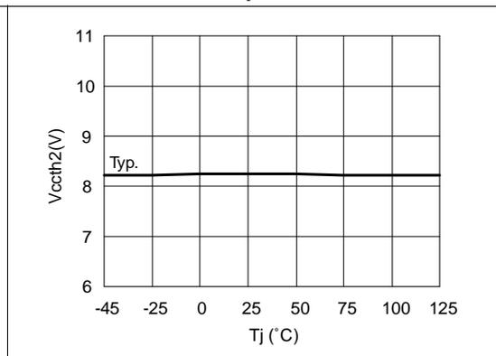
**Figure 10. V<sub>BOOT</sub> UV turn-off threshold vs. temperature**
