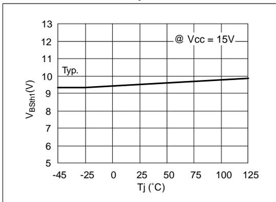
**Figure 9. V<sub>CC</sub> UV turn-off threshold vs. temperature**
