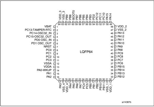
Figure 4. STM32F100xx value line LQFP64 pinout
