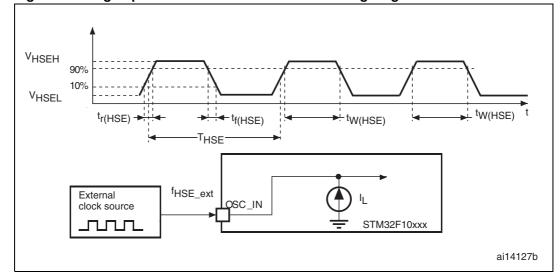
Figure 18. High-speed external clock source AC timing diagram
