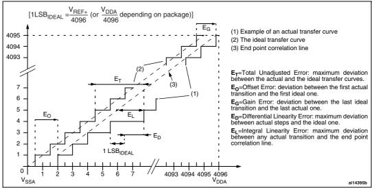
Figure 32. ADC accuracy characteristics
