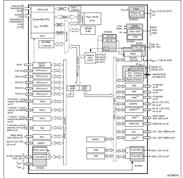
Figure 1. STM32F100xx value line block diagram
