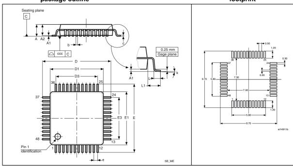
Figure 43. LQFP48 – 7 x 7 mm, 48-pin low-profile quad flat Figure 44. Recommended package outline<sup>(1)</sup> footprint<sup>(1)(2)</sup>
