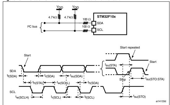
Figure 28. I<sup>2</sup>C bus AC waveforms and measurement circuit<sup>(1)</sup>
