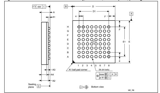
Figure 41. TFBGA64 - 8 x 8 active ball array, 5 x 5 mm, 0.5 mm pitch, package outline
