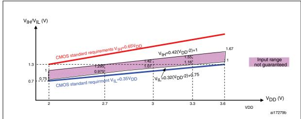
Figure 24. 5 V tolerant I/O input characteristics - CMOS port
