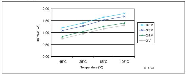
Figure 15. Typical current consumption in Stop mode with regulator in Run mode versus temperature at  $V_{DD}$  = 3.3 V and 3.6 V
