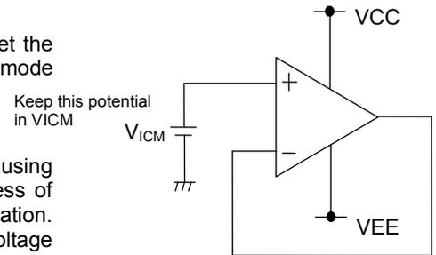
Figure 100. Example of Application Circuit for Unused Op-amp
