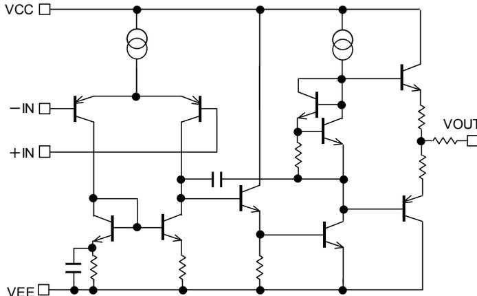
Figure 1. Simplified Schematic
