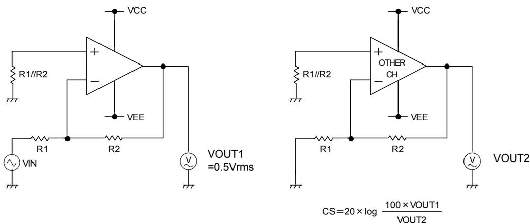
Figure 93. Test Circuit 3(Channel Separation)
