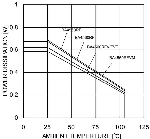
Figure 24. Derating Curve
