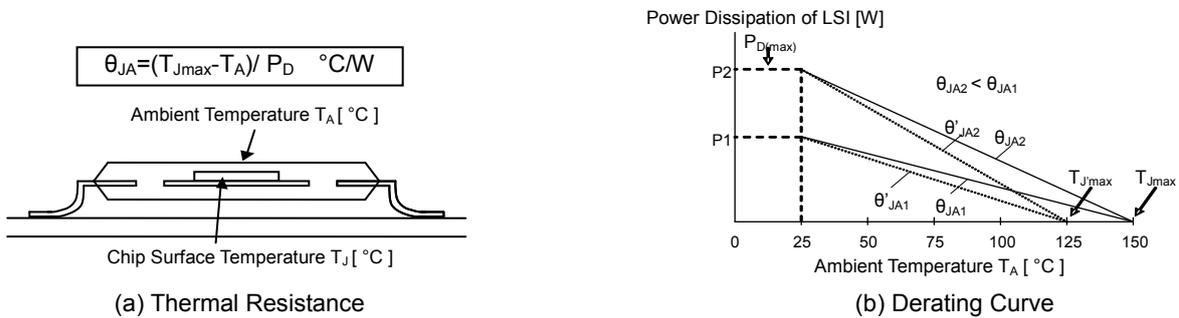
Figure 94. Thermal Resistance and Derating Curve
