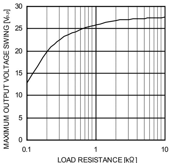
Figure 27. Maximum Output Voltage Swing - Load Resistance (VCC/VEE=+15V/-15V, T<sub>A</sub> =25°C)
