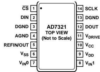
Figure 3. Pin Configuration
