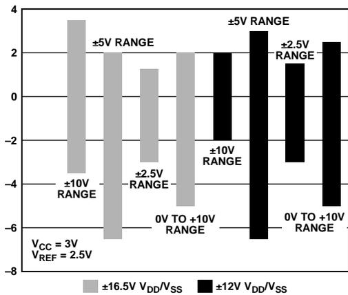
Figure 41. Pseudo Input Range with  $V_{CC} = 3V$
