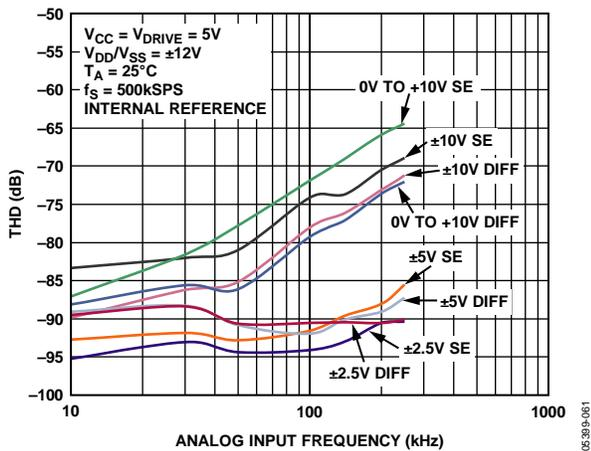
Figure 11. THD vs. Analog Input Frequency for Single-Ended (SE) and True Differential Mode (Diff) at 5 V<sub>CC</sub>
