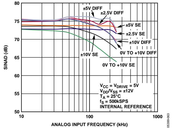
Figure 13. SINAD vs. Analog Input Frequency for Single-Ended (SE) and True Differential Mode (Diff) at 5 V<sub>CC</sub>
