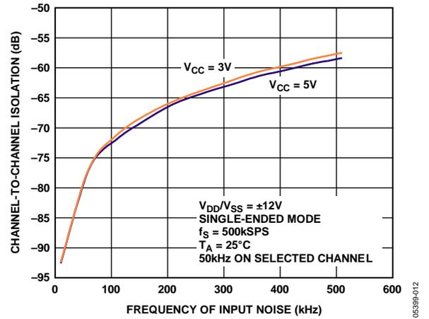
Figure 14. Channel-to-Channel Isolation
