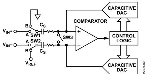
Figure 26. ADC Differential Configuration During Conversion Phase
