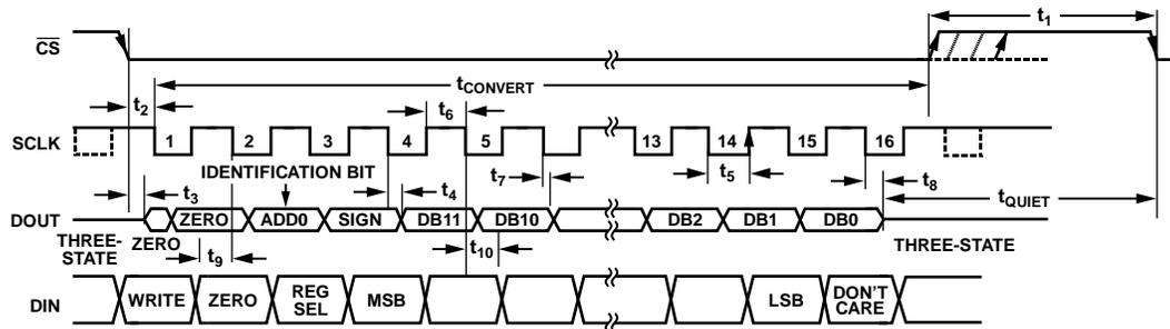
Figure 50. Serial Interface Timing Diagram (Control Register Write)
