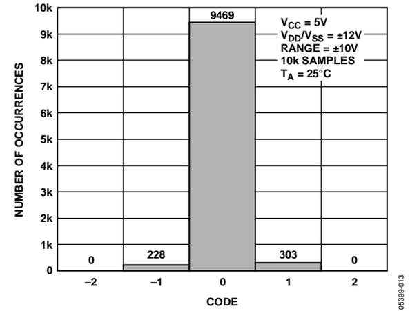
Figure 15. Histogram of Codes, True Differential Mode
