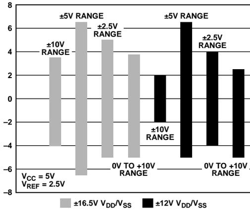
Figure 40. Pseudo Input Range with  $V_{CC} = 5V$
