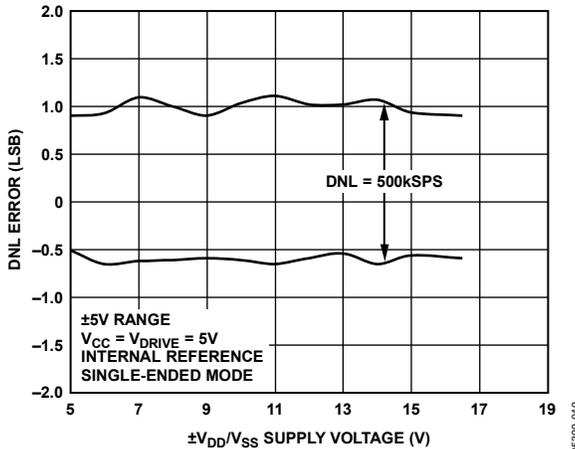
Figure 18. DNL Error vs. Supply Voltage at 500 kSPS
