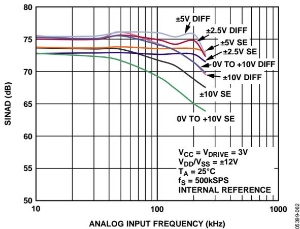
Figure 12. SINAD vs. Analog Input Frequency for Single-Ended (SE) and True Differential Mode (Diff) at 3 V<sub>CC</sub>
