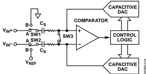
Figure 25. ADC Differential Configuration During Acquisition Phase
