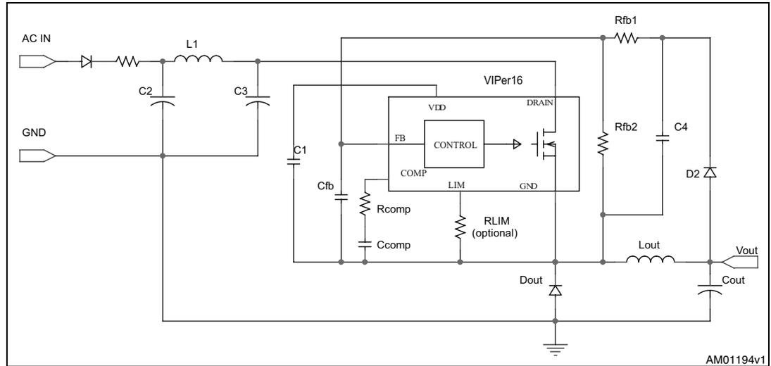
**Figure 18. Buck boost converter**
