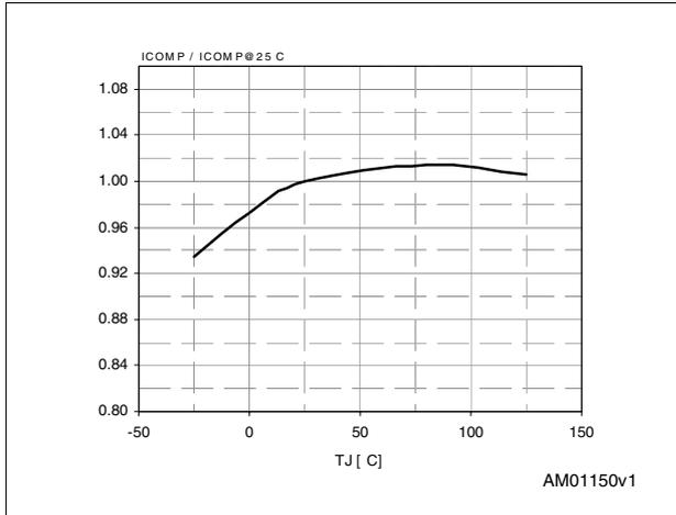
Figure 11. Operating supply current (no switching) vs  $T_J$
