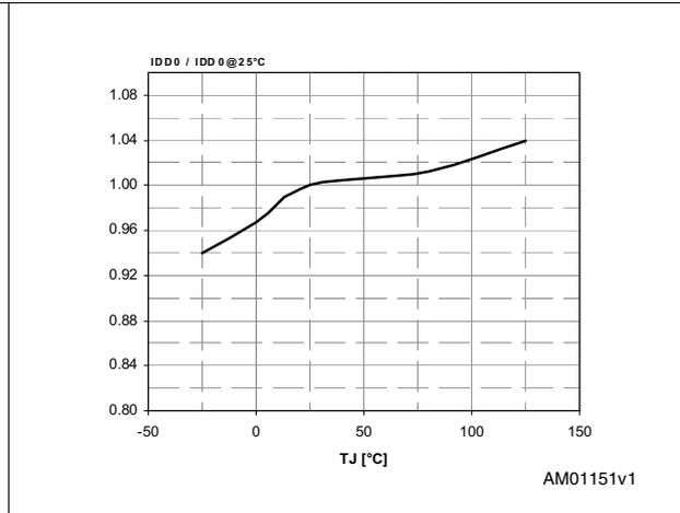
Figure 12. Operating supply current (switching) vs  $T_J$
