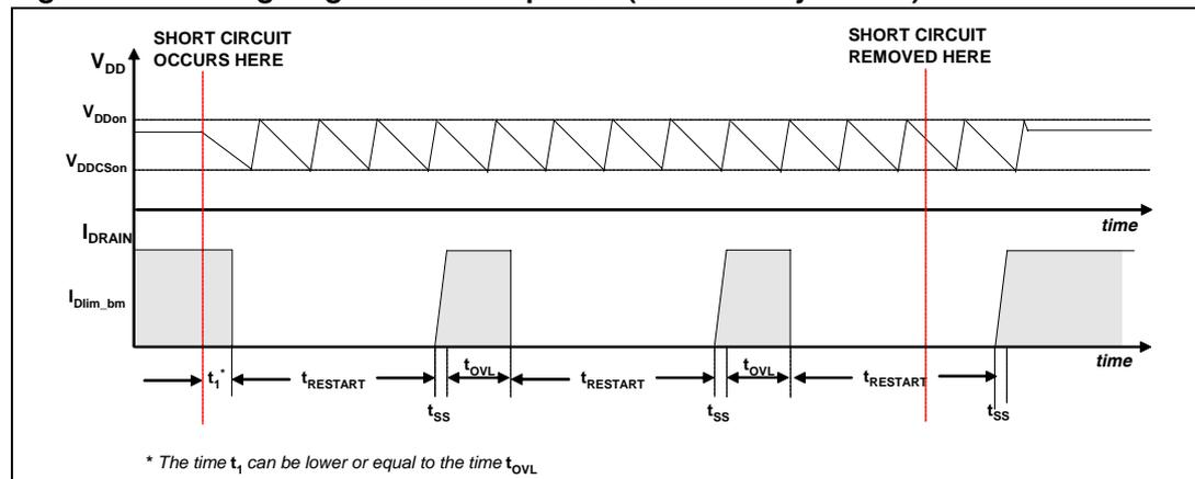
**Figure 26. Timing diagram: OLP sequence (IC internally biased)**
