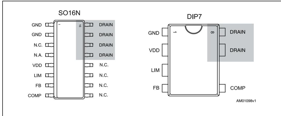
Note: The copper area for heat dissipation has to be designed under the DRAIN pins.
