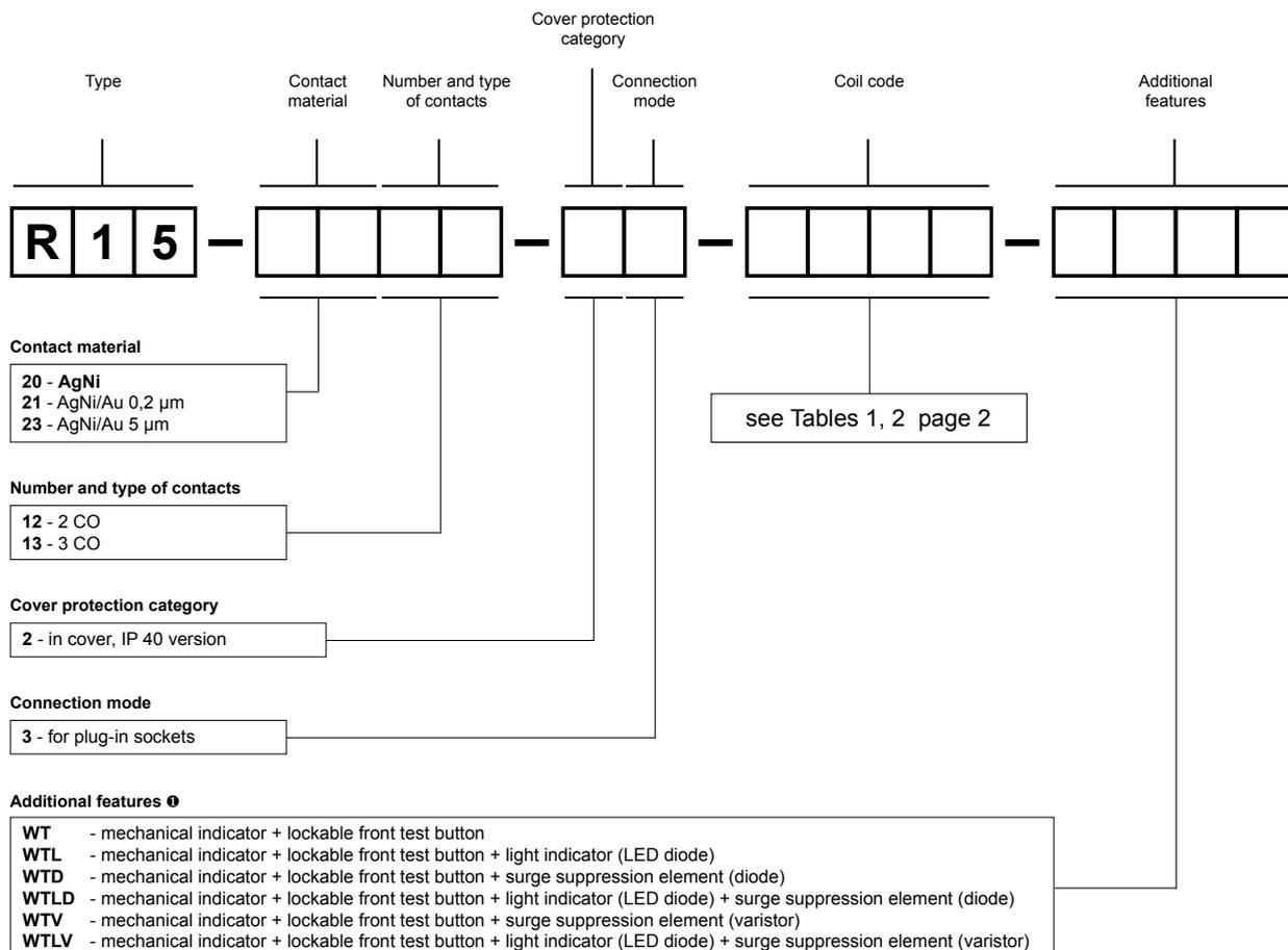
❶ **WT** - standard features of relays for plug-in sockets. **WTD, WTL D** - only for DC coils, **WTV, WTLV** - only for AC coils
