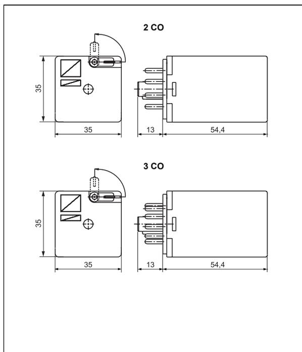
**Dimensions - plug-in version, with test button
