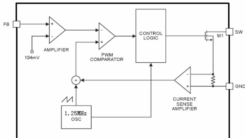
Figure 3. Simplified Block Diagram of the PT4101
