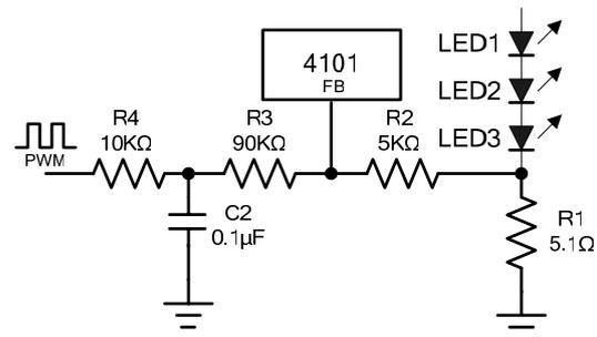
**Figure 6. Dimming Control Using a Filtered PWM Signal**
