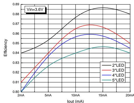
Figure 2. Efficiency vs Number of LEDs
