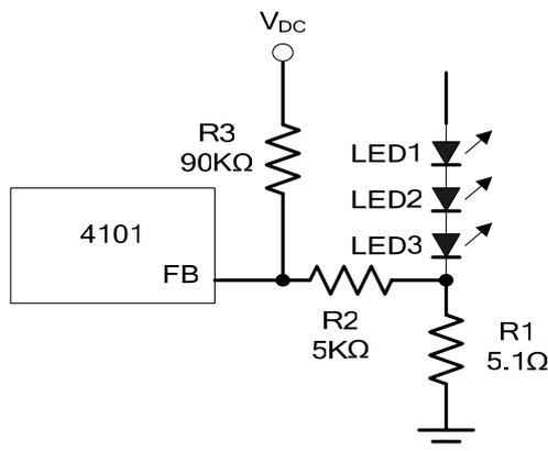
**Figure 4. Dimming Control Using a DC Voltage**
