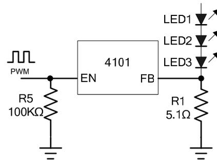
**Figure5. Dimming Control Using a PWM Signal**
