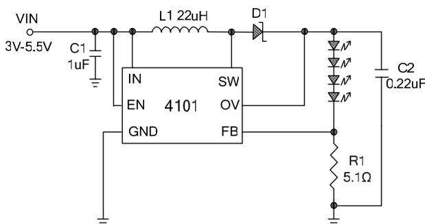
Figure 1. Li-Ion Driver for Four White LEDs
