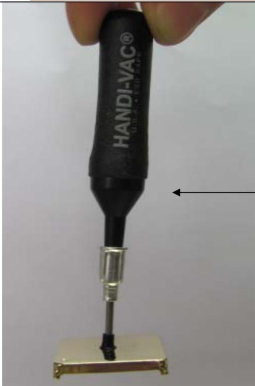
The experimental result: 1/8" (3.18mm) diameter vacuum cup draws a maximum weight of 1.4 g.
