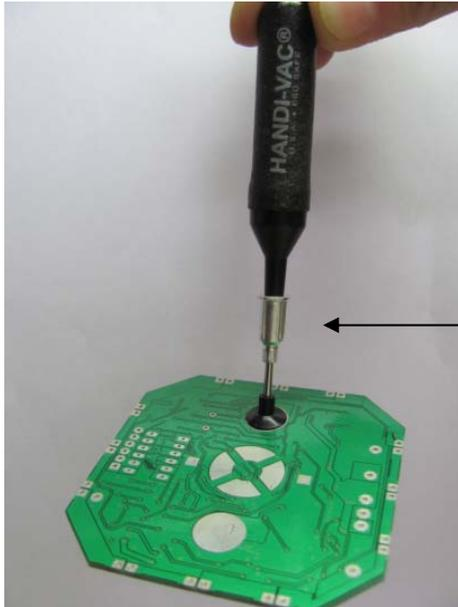
The experimental results: 3/8" (9.53mm) diameter vacuum cup draws a maximum weight of 13 g.
