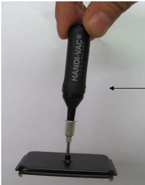
The experimental result: 1/4" (6.35 mm) diameter vacuum cup draws a maximum weight of 5.8 g.
