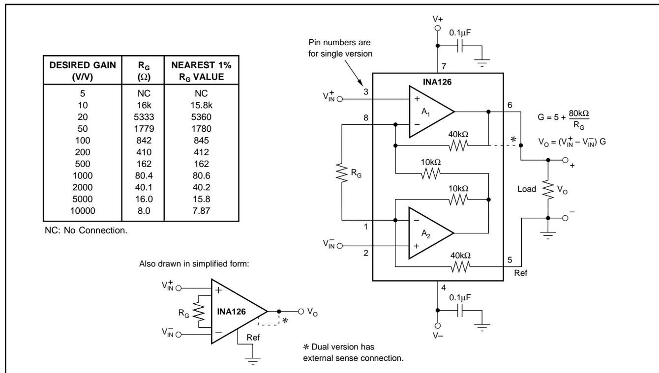
FIGURE 1. Basic Connections.
