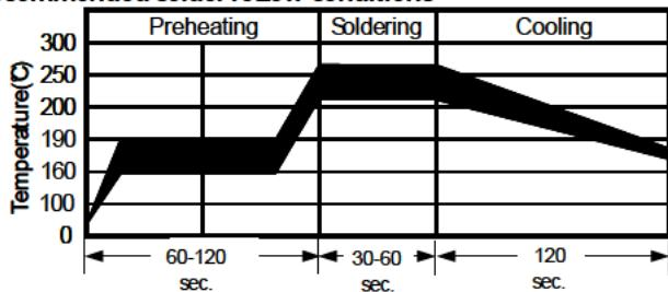
Recommended reflow methods: IR, vapor phase oven, hot air oven.
