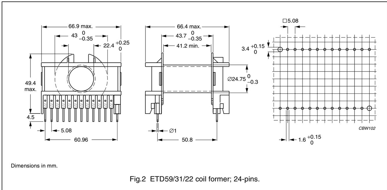
**Winding data and area product for 24-pins ETD59/31/22 coil former**
